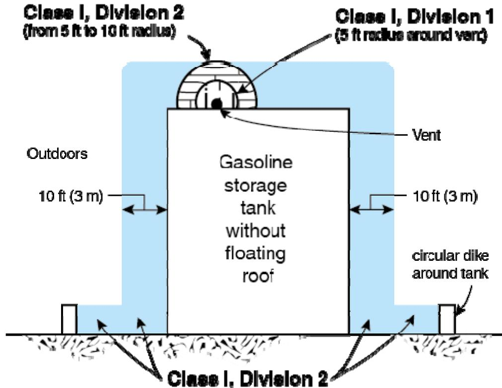
The picture above is an example of a typical classification of a fuel storage tank.
