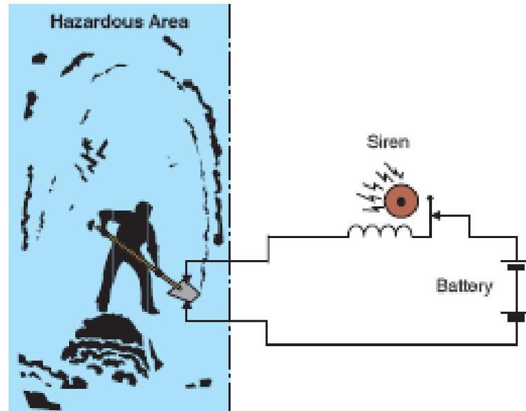
Research, however, revealed that ***the most important factor in determining the safety of an electrical circuit is the energy stored in the circuit.*** Without the use of limitation methods, the inductive energy stored in the bell and wiring produced energy levels sufficient enough to generate an electric arc that was able to ignite the dangerous air/gas mixture.
