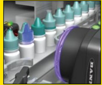
Checking the integrity of tamper-evident seals by verifying both presence and correct position.
