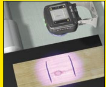
Sensing fluorescent markings for wood defects on timber material even at long sensing distances.
